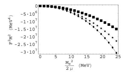
Figure 2: Squared mass of the kaon modes times  $F^2$ , in the neutral CFL phase with massless u and d quarks, against  $M_s^2/2\mu$ . Diamonds and stars correspond respectively to  $\Delta = 25 \text{ MeV}$  and  $\Delta = 75 \text{ MeV}$ . Squares correspond to the leading order solution, which does not depend on  $\Delta$ . In the figure we have chosen  $\mu = 500 \text{ MeV}$  as a reference value of the baryon chemical potential.
